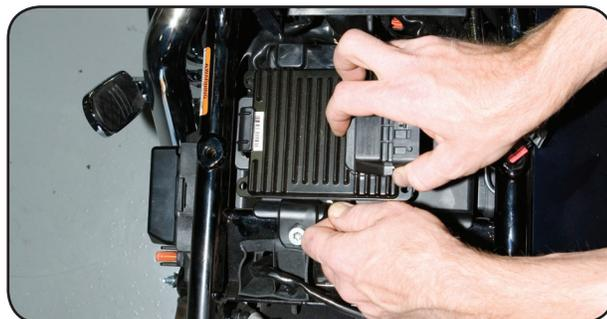
2. Remove ECU by pushing tab and sliding the ECU to the right as you lift.
