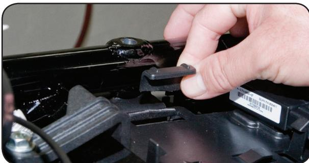
3. Cut and remove the left ECU hold down to allow the ECU to slide over.
