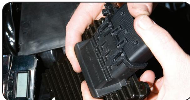
4. Gently align the pins of the Fuelpak connector with the ECU and press the connector on the ECU. Be sure the single large pin is aligned with the single large socket before pressing Fuelpak connector into the ECU. Make sure all four tabs fully latch. (Fuelpak connector Patent Pending# 29 295831)
