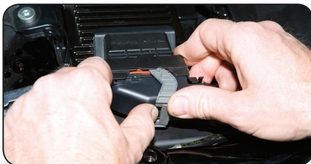
1. Remove seat, exposing factory computer (ECU), disconnect factory wiring by pressing lock and pushing lever back.
