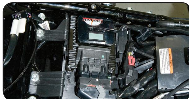
7. Attach Fuelpak to the top of the ECU by using the supplied Velcro.
